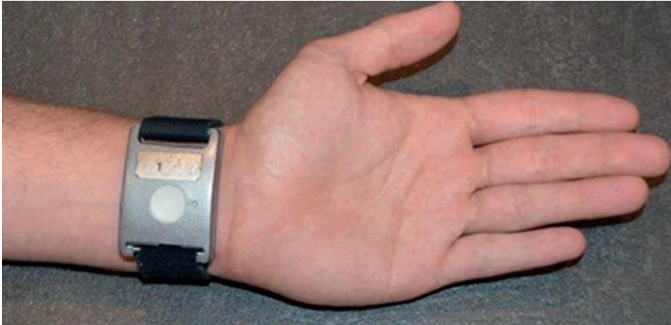
FIGURE 1. Photograph of a Q-sensor used to assess the skin conductance levels of staff members during a day, evening, and night shift.
